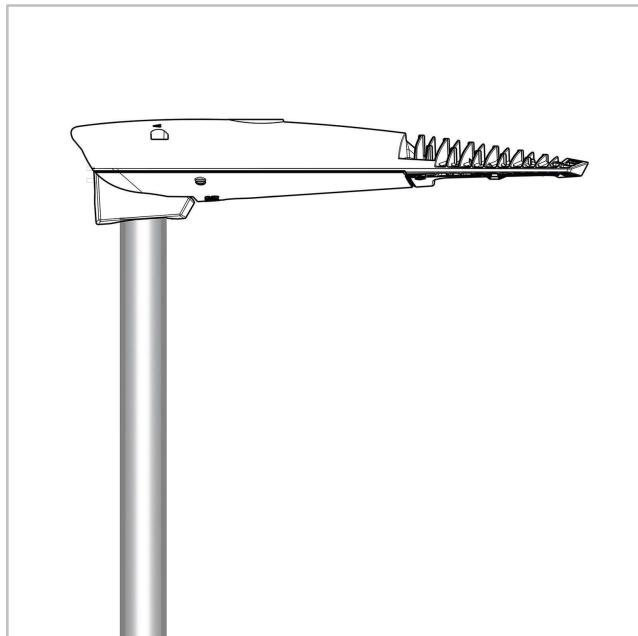
AXIA 2 | Post-top - Slip-over mounting for Ø60 or Ø76mm spigot - 2xM10 screws
